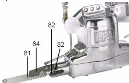
Figure 3: Loosening the sawblade
